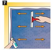
For extra lubrication spray more **Application Solution**. Starting from top-centre, use **Applicator Tool** to work out bubbles to edges.
