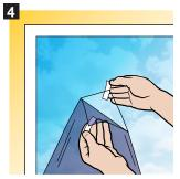
Peel away backing by placing a small piece of masking tape front and back on 1 corner of film and separate.
