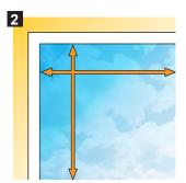
Measure width and height of glass area to cover using a metal tape measure for accuracy.
