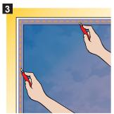
On a clean flat surface, cut window film 20-25mm wider than required along all sides to ensure coverage.
