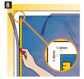
Using a Straight Edge, trim excess film leaving a 1-2mm gap for any water residue to escape.
