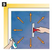
Lightly spray with more **Application Solution** and work out any remaining bubbles. Use cloth to capture excess moisture.
