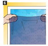
Place adhesive side of film against glass and gently manoeuvre film into position. Smooth out bubbles by hand.
