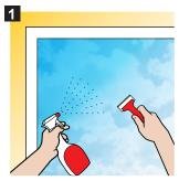
Thoroughly clean glass to remove all dirt and debris using an ammonia-free cleaner, scraper & lint-free cloth.
