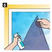
Apply a generous amount of **Application Solution** to glass and **BOTH** sides of window film to allow for easy installation.
