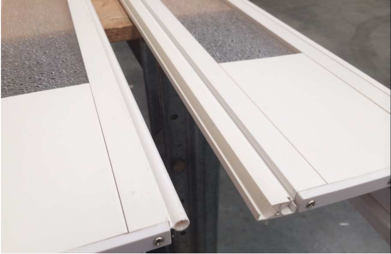
4. Door is now ready to have panels added.
